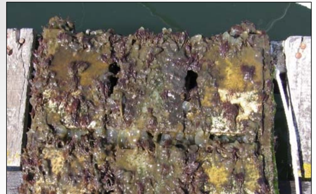
Control panels, 30 days immersion
