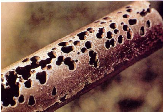
MIC damage: heat exchanger pipe (Al) (van Pelt, 2006)
