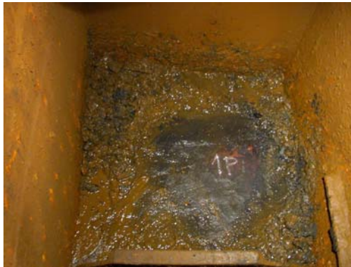
MIC damage: uncoated (left) and coated (right) ballast tanks (TNO survey, 2006)
