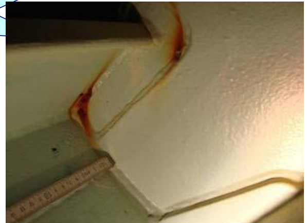
Hr.Ms. "Tromp" (LCF 2). Potable water tank 4: Corroded spots along welds.
