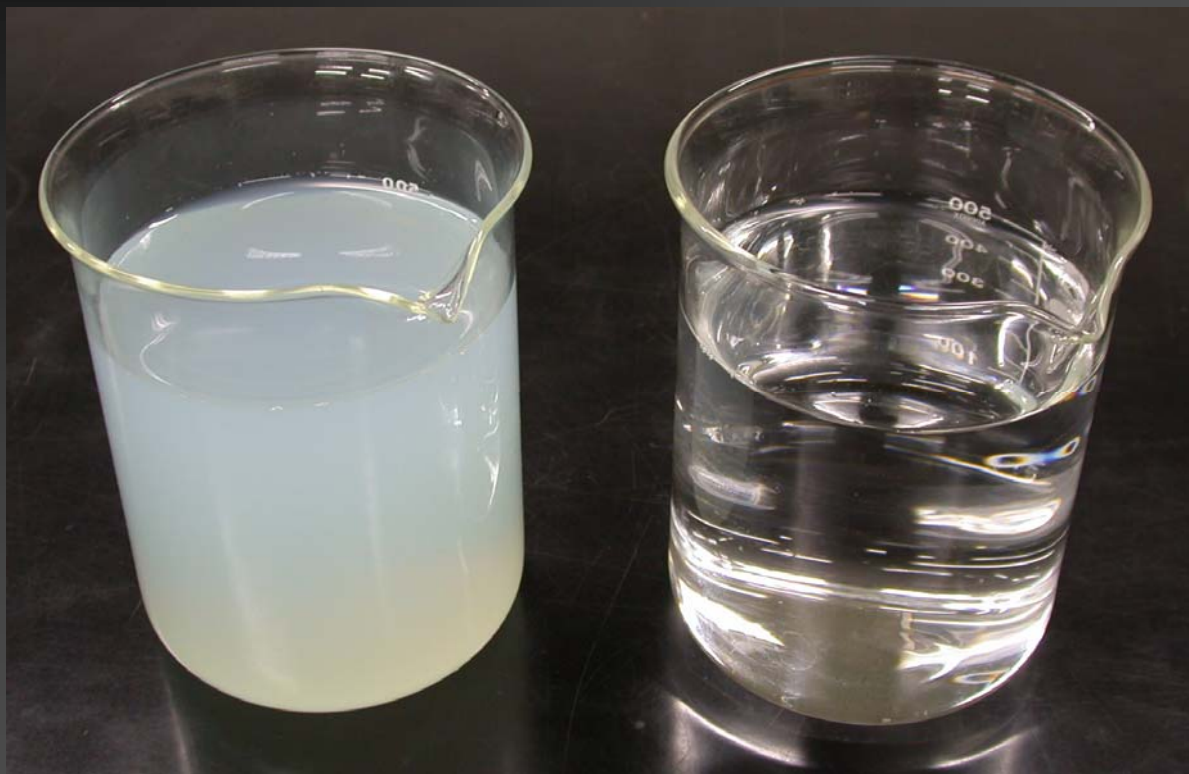
Copper added into natural seawater at 10 mg-Cu/L
