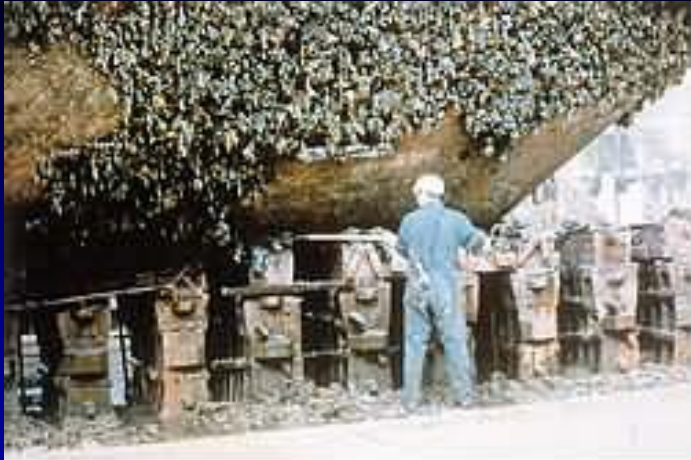
Ship in dry dock with fouled hull.
