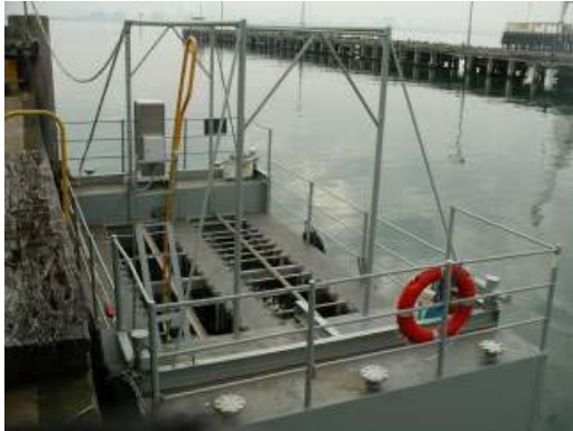
Static immersion trials in southern and northern Australia
