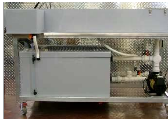
Flow chamber to evaluate adhesion strength and foul-release capabilities
