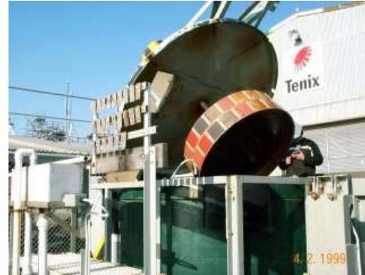
Rotor facility to evaluate coating durability
