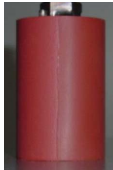
Rotor sand-blasted + application of an anticorrosive coating
