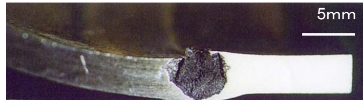
Stainless steel welds attacked by MIC
